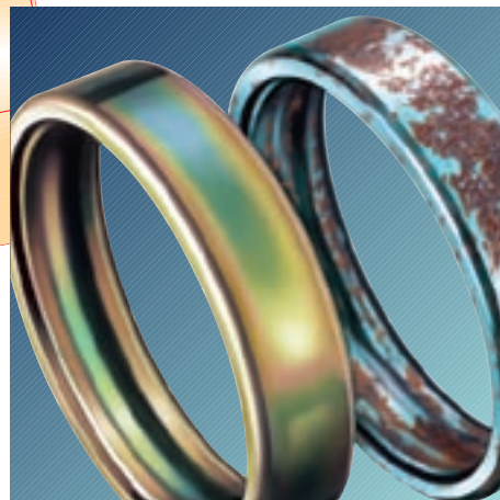
Compare for yourself: Corrotect®-plated part and unplated part after a two-hour salt spray test
