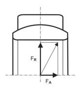
Figure 7: Radial and axial force
