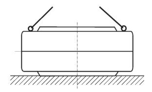
Figure 6: Transporting large spherical plain bearings
