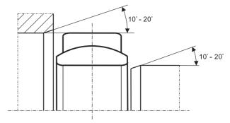
Figure 2: Centering chamfers
