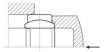
Figure 5: Combination installation tool
