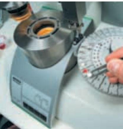
DSC analysis: Temperature behavior of lubricants, analyzed using the latest methods
