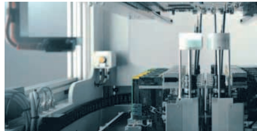
Dynamic, precise, maintenance-free: Planar system in flying probe testers
