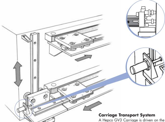
horizontal slide by a friction drive.
