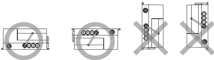
(If the vertical installation is required, please turn batteries in a box upwards to avoid short circuit.)
