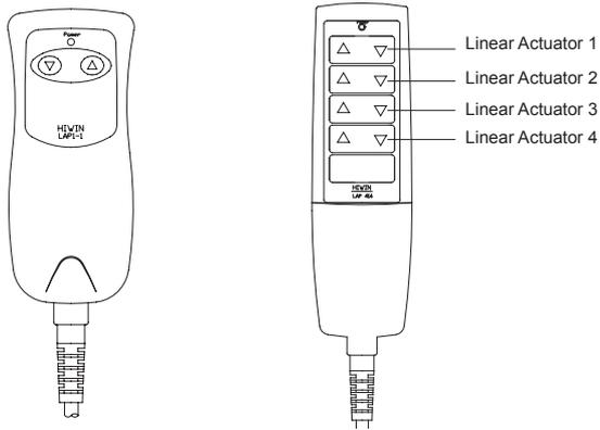
2. When you press the “△” key, the extension tube of actuator will extend outward (see a figure below).
