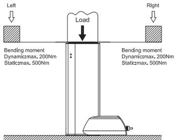
3.3. For fixing the extension tube in this actuator on one guiding mechanism, please refer to the installation guide. If it is not fixed on any mechanism, it could idle.
