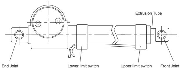
※ If an actuator doesn't have an external limit switch installed, you must install the stroke limiter on an actuator yourself. The distance between two actuator limit switches can't be longer than the stroke of the actuator. And then rotate the extension tube to adjust the length of an actuator, which can meet the minimum requirements to install actuators.
