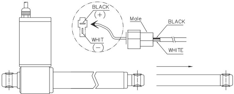
3.4 When the input power is reversely connected (wiring as a figure below), the inner tube of actuator will draw inward.
