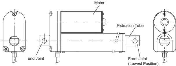
2.1.2 External limit switch: For installing an external limit switch, please ensure the extension tube is in the lowest position before installing an actuator (Please refer to the figure below.).
