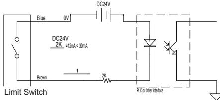
2. High-level Control (taking PLC for example)
