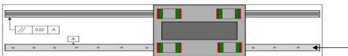
Figure 4.8: Installation of the travel block on the guide rails
