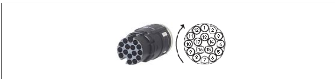
Figure 5.6: PIN assignment of the round connector for the distance measuring system (looking down onto the axis)
