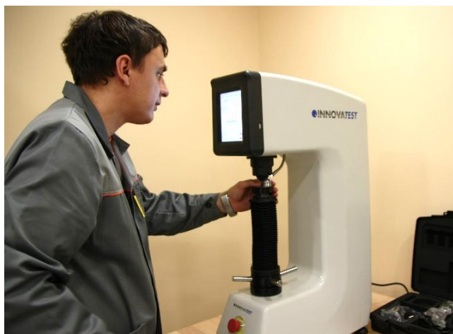
Twardościomierz INNOVATEST NEXUS 610 RSB (INNOVATEST Europe BV, Niderlandy)
