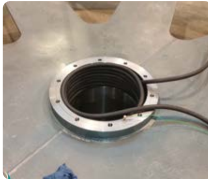
Heating a bore for bearing or shaft mounting
