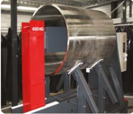
BETEX GIANT Adapted for heating large stainless steel pipes (1100 kg), used in wind turbines.
