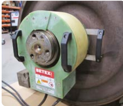
Heating bearing rings for dismounting
