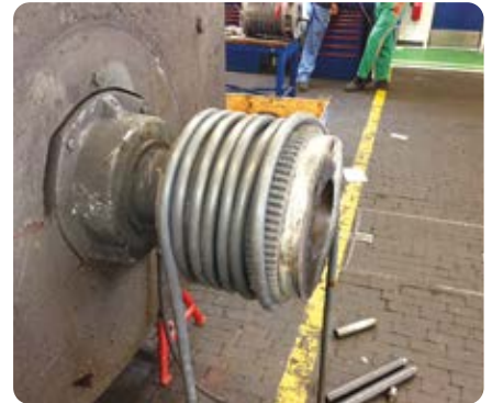
Heating a coupling for dismounting
