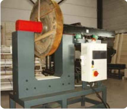
BETEX GIANT Adapted for heating train wheels. The induction yoke is extendable.
