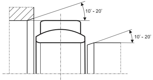
Figure 2: Centering chamfers
