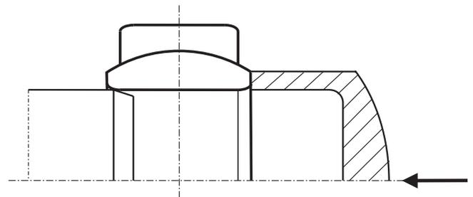
Figure 3: Installation tool
