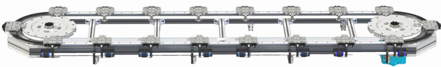
There is no fundamental limit to the number of carriages that can be used in a configuration, but the loads applied to the belt and belt connection will generally be the factor which determines the most appropriate system size for an application. The linear speed and rate of acceleration will affect the load on the belt connections and torque through the drive assembly.
