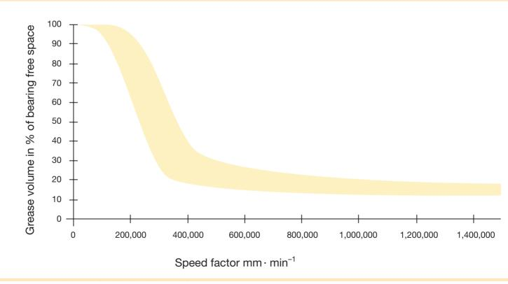
Grease fill as a function of the speed factor
