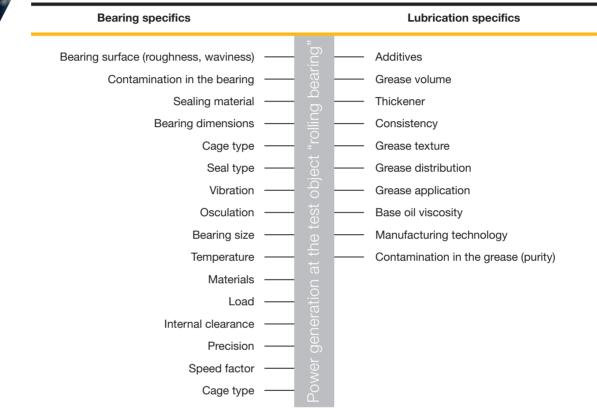
Both mechanical and lubrication-related factors can jointly influence the particular operating noise level of a rolling bearing. The combined noise behavior of the rolling bearing and lubricant is measured on special noise test equipment. It is often difficult to identify which influencing factors are responsible for generation of both solid and air-borne sound.
