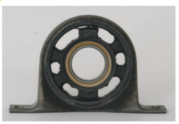
Drive shaft support - Messrs. Vibracoustic
