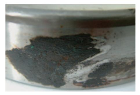
Fretting corrosion on the outer ring
