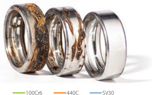
Test Results from Salt Spray Test according to DIN 50021 / ASTM B117-7
