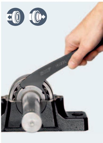
Easy and quick bearing mounting and dismounting in SNL housings
