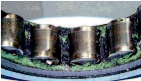
Lubricant degradation caused by electrical discharge currents
