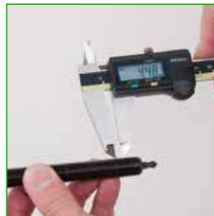
c Measure the length over three turns of the thread.
