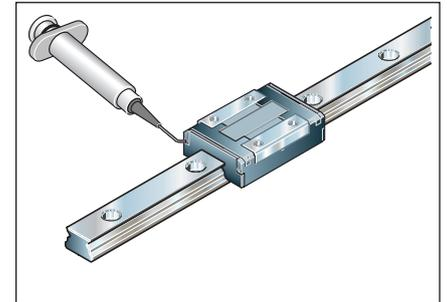
If the **funnel-type lube nipples** on the runner block end faces are preferred, use a **grease gun** instead.
