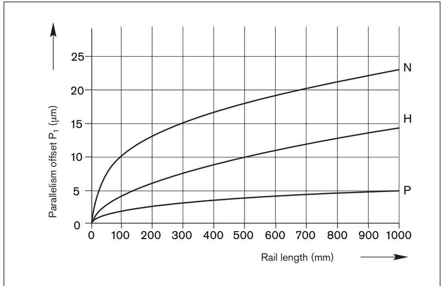
**Parallelism offset of the installed rails measured on the guide rails and on the runner blocks**
