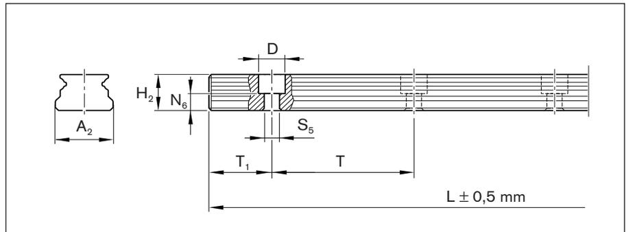
Position tolerance of the mounting holes for
