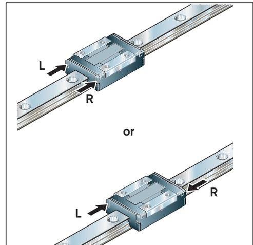
For **short stroke** applications, apply the partial amount per side as given in the table to each end-face lube port.
